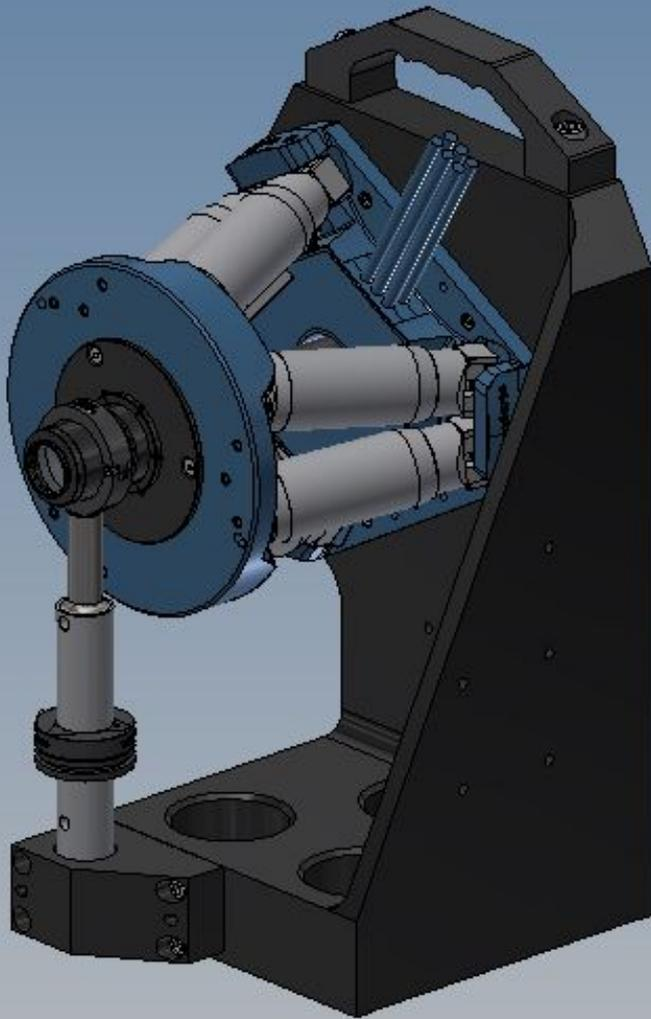
Fold mirrors clearing IM and ASM path
