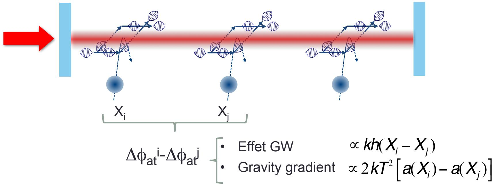
Discrimination between GW effects and gravity gradients using the spatial resolution of the antenna
