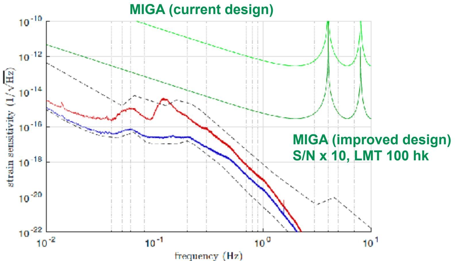
MIGA strain sensitivity. In blue (resp. red) seismic GGN projection from Lsbb 50th percentile of a quiet week (resp. 90th percentile of a noisy week), in dashed black from Peterson model data, in green detection noise for MIGA in its initial configuration (light green) and for an improved version (dark green).
