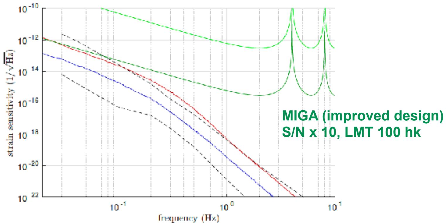
MIGA strain sensitivity for the infrasound GGN, with data from Bowman model (dashed black) and from data gathered on site at the Lsbb (50th percentile in blue and 90th percentile in red).
