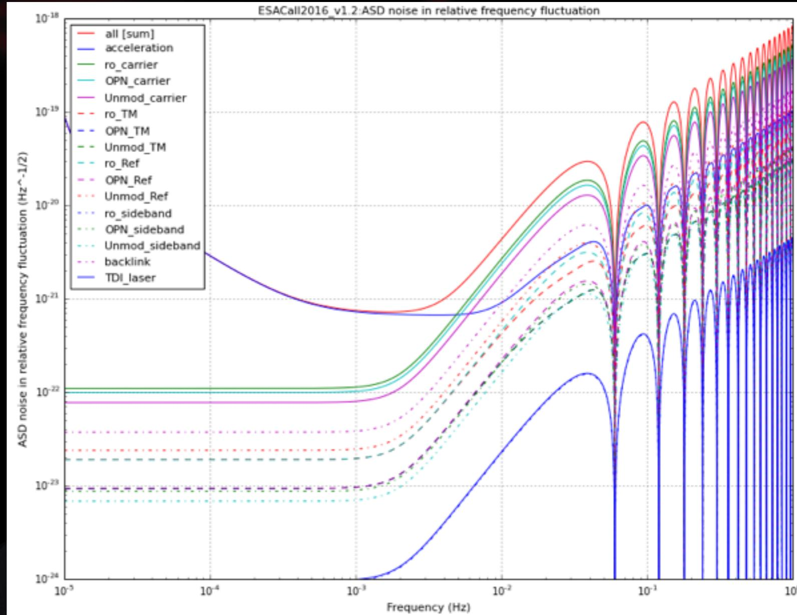
$$S_a^{1/2} \leq 3 \cdot 10^{-15} \frac{\text{m s}^{-2}}{\sqrt{\text{Hz}}} \cdot \sqrt{1 + \left( \frac{0.4 \text{ mHz}}{f} \right)^2} \cdot \sqrt{1 + \left( \frac{f}{8 \text{ mHz}} \right)^4}$$
