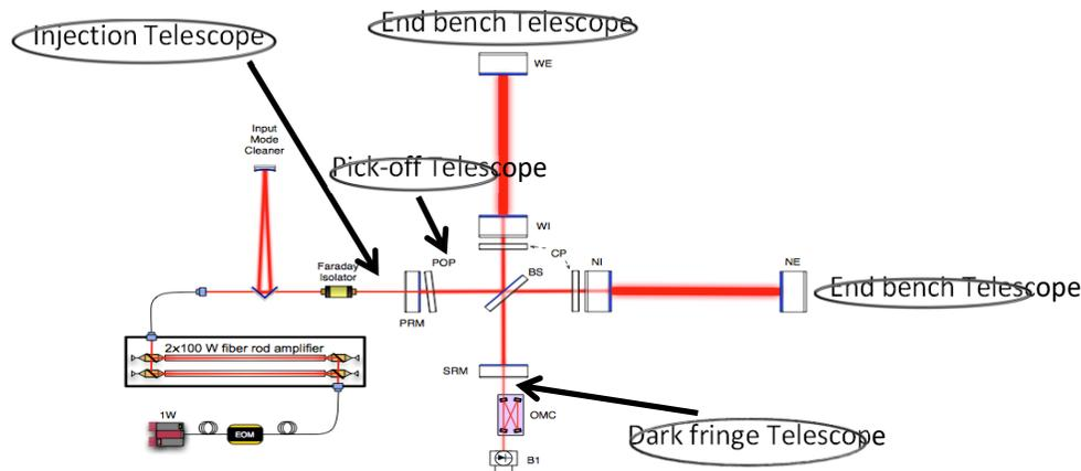
**End benches example:** diffused light produces a change in the phase inside the FP cavities which mimic a GW
