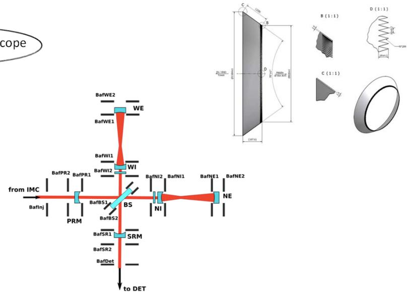
Figure 9.12: Layout of the baffles suspended to the Super Attenuators.
