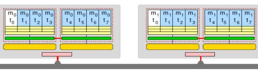
One MPI process / socket: OpenMP threads on same socket: "blockwise"
