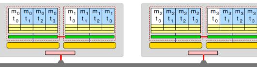
OpenMP threads pinned "round robin" across cores in node
