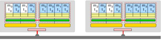
Two MPI processes / socket OpenMP threads on same socket
