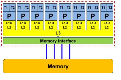
Intel Xeon "Sandy Bridge EP" socket 4,6,8 core variants available Floating Point (FP) Performance:  $P = n_{core} * F * S * v$ 8 number of cores: **n**<sub>core</sub> FP instructions per cycle: 2 (1 MULT and 1 ADD) **FP ops / instruction:** 4 (dp) / 8 (sp) (256 Bit SIMD registers – "AVX")
