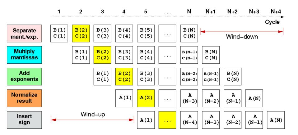
First result is available after 5 cycles (=latency of pipeline)! Wind-up/-down phases: Empty pipeline stages
