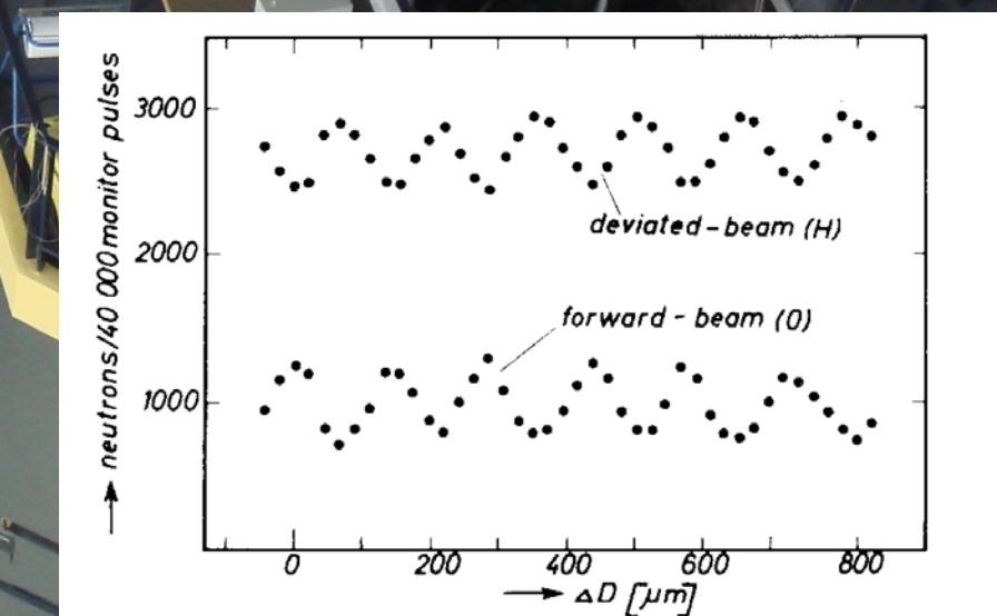
Fig. 2. Measured intensity modulation of the deviated and forward beam as a function of the different optical paths for beam I and II within an Al-sheet. (The statistical error is smaller than the size of the points.)
